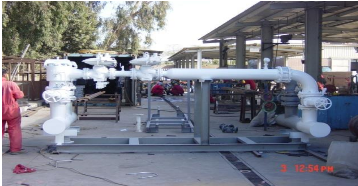
Regulator Station Under Fabrication 5000 m 3 /hr
