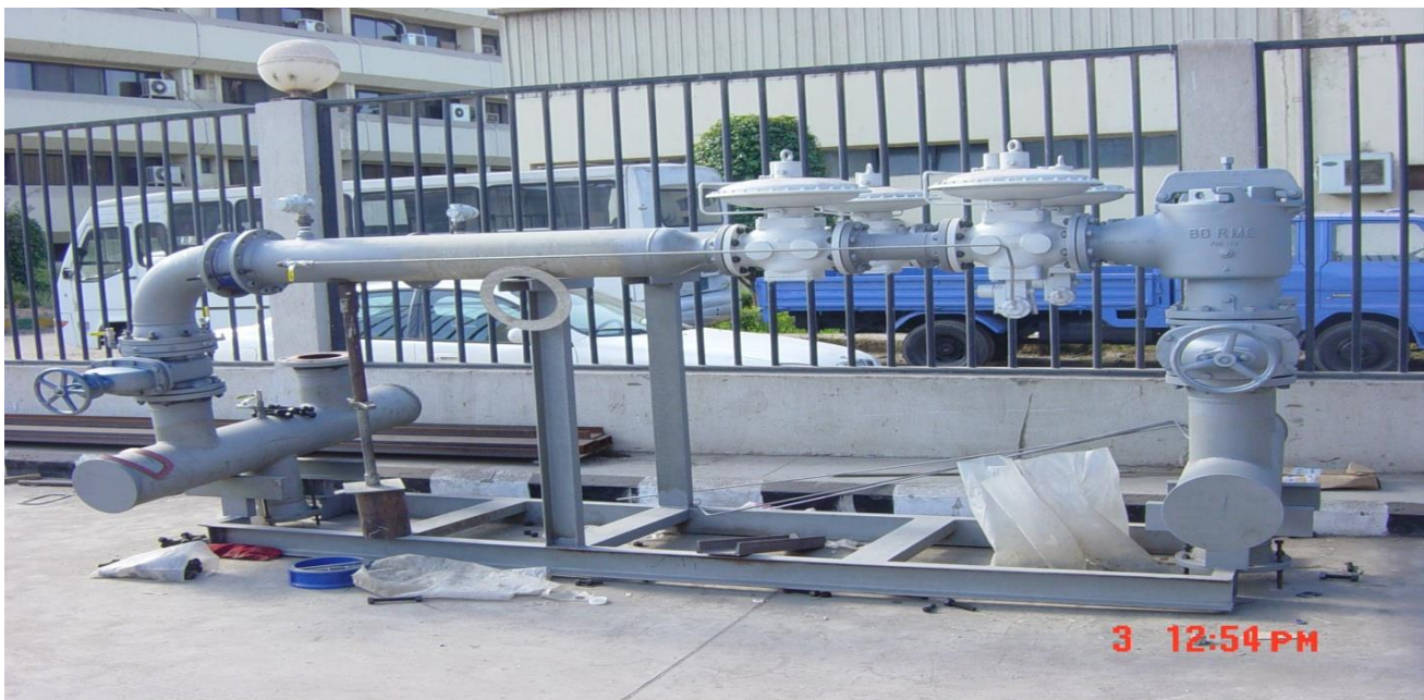
Regulator Station Under Fabrication 5000 m 3 /hr
